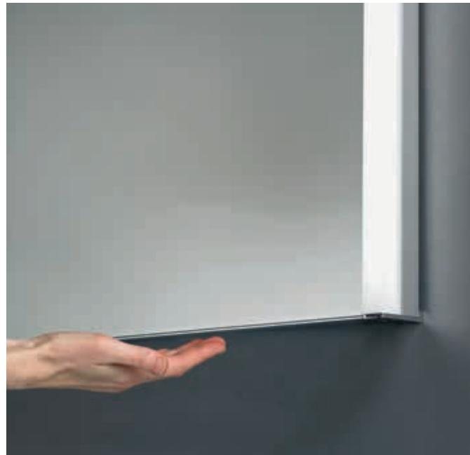
The frame 25 mirrors can be fitted with a touch sensor on the frame. It switches the LEDs on and off, and causes them to dim. These LEDs light up the washbasin area homogeneously and with daylight quality light: That means that colours are displayed naturally, and the individual LED points cannot be detected.
