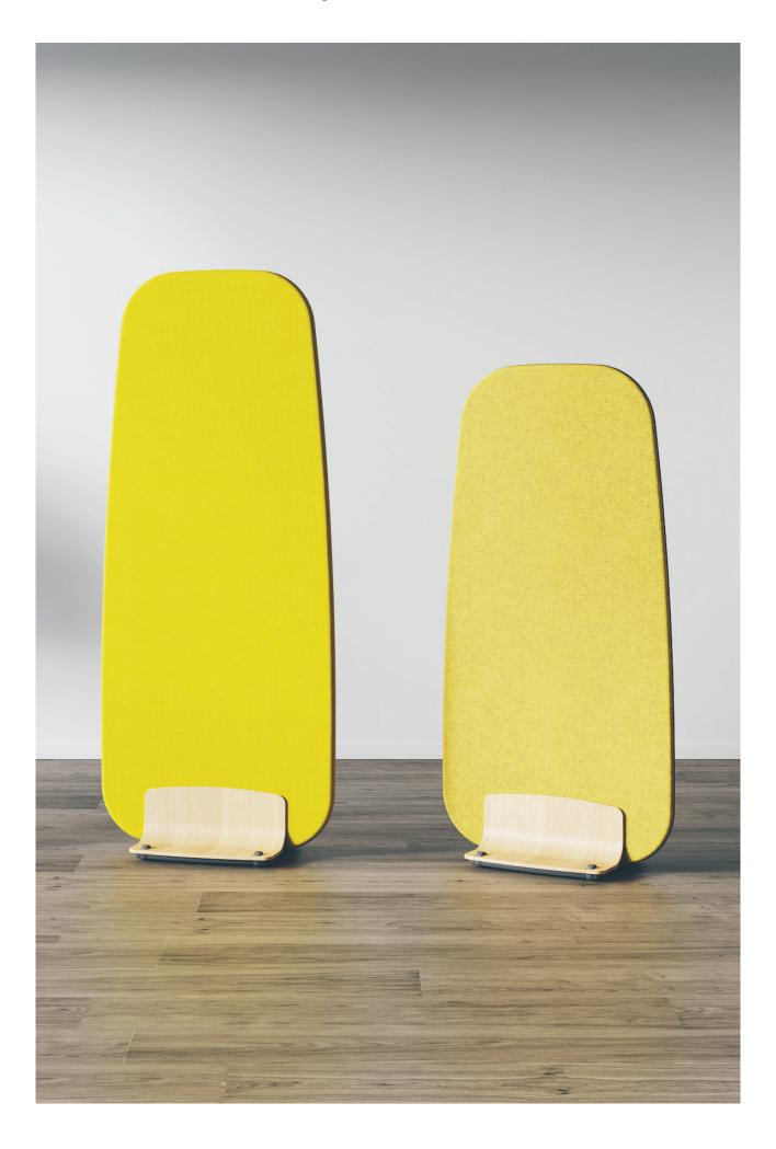
This sound absorbing floor screen has optional write board. Frame: 6 mm sound absorbing polyether (Oeko-Tex) glued on both sides of a 19 mm sound reducing lightweight MDF. Writing board: 4 mm writing board in white glass with magnetic back. Pen strip: Solid ash with integrated eraser and magnets. Upholstery: Furniture nailed with fabric on both sides. The nail is hidden by a decorative piping. Wheel stand in ash natural or stain.
