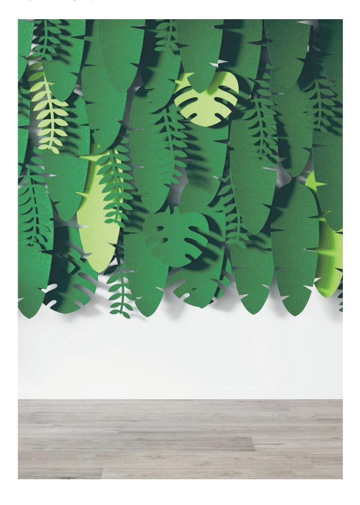
JungleWall is a series of sound absorbent leafs in different patterns. The material is made of felt and the leafs can be mounted in a way that creates a distance to the wall. The material in JungleWall, along with the distance to the wall, creates a good condition for sound absorption. Leaf: 5 mm polyester felt, hook: solid ash. 100% recyclable material.
