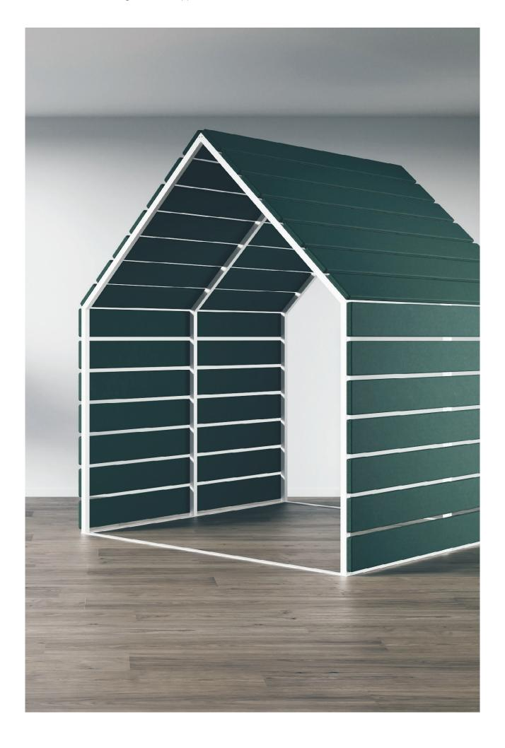
LimbusBarn 270 has a white metal frame in 40 mm square tubes which stands on a frame in flat iron. The parts are coupled with hidden connection angles. 28 panels that form walls and roof are hooked onto the frame. Panels: 19 mm Lightweight MDF with 6 mm polyether and fabric. Matching colours in fabric piping. Metal frame: Powder coated NCS S 0500-N White. 100% recyclable material.
