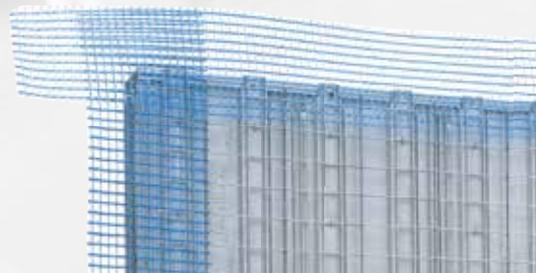
*Frames are supplied complete with a special plastering mesh. Fixed to the edges of the metal box where it meets the wall, this mesh protects against cracking of the plasterwork. This special mesh in fibreglass has been chosen because it is suitable for walls of all types, is easy to use and offers excellent resistance, thanks to its particularly tight structure.*
