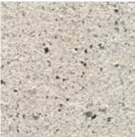
sandblasted surface with granite aggregates
