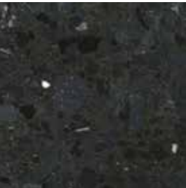
polished surface with black marble aggregates
