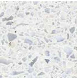
polished surface with white marble aggregate
