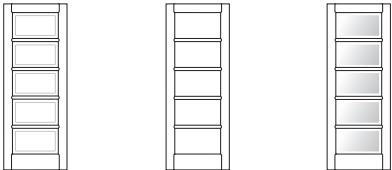
cieca con bugna blank with raised panel cieca con foderina blank with flat panel finestrata glazed
