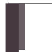
Porta scorrevole esterno muro composta Outside the wall sliding door with two overlapping double leaves
