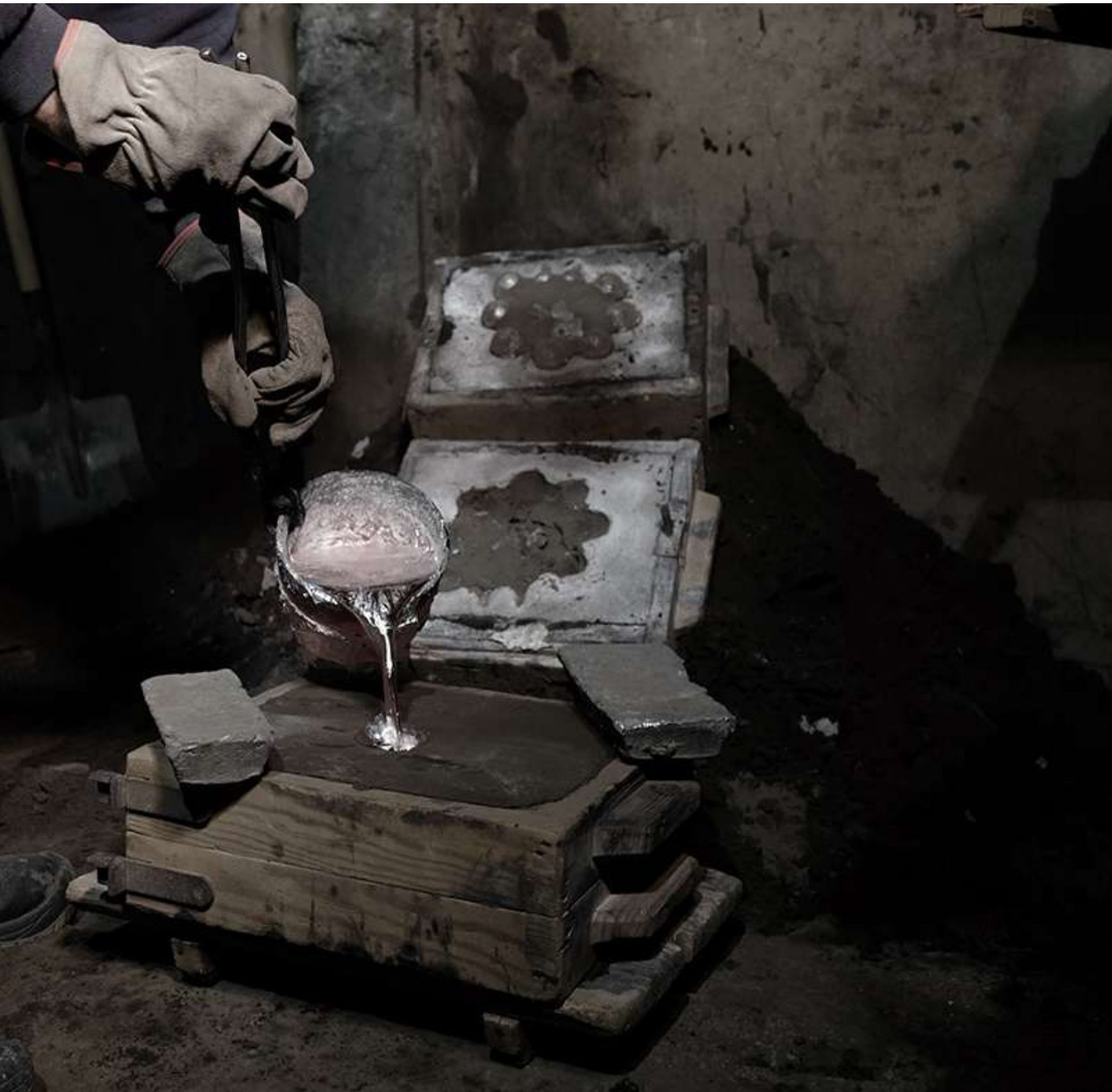
Metal casting starts with melting metal into a liquid, pouring it in a mold with a cavity of the desired shape
