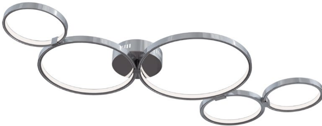
▲ MOD448-44-N LED 30W H: 70, W: 740, L: 440 mm, 1500 Lumen, 3000 K, 80 RA, 120 °, 220-240 V, IP20
