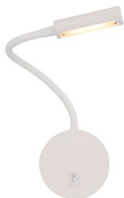
C035WL-L3W3K ⚡ LED 3W H: 470, W: 31, L: 100 mm, 150 Lumen, 3000 K, 80 RA, 120 °, 220-240 V, IP20, Class 2,
