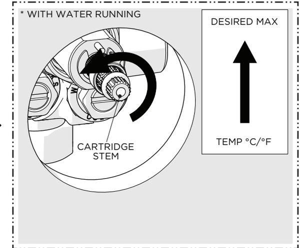
14. With water running, rotate the STEM to adjust the temperature to the **maximum** desired bathing temperature, verified with a thermometer, then close the VOLUME CONTROL VALVE and make sure **NOT** to change this setting.
