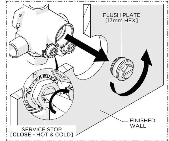
1. Turn on the water supplies then remove the TILE GUARDS from the VALVE and **OPEN** the SERVICE STOPS (hot & cold) and **INTEGRATED VOLUME CONTROL VALVE** to flush out the lines.
