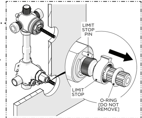
**IF THE MAXIMUM BATHING TEMPERATURE IS NOT CORRECT OR NEEDS TO BE ADJUSTED:**
