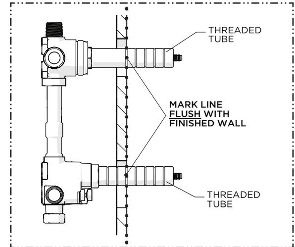
5. Mark both TUBES where they protrude past the finished wall.
