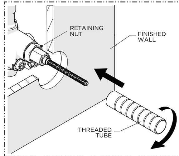
4. Thread the THREADED TUBE into the RETAINING NUT until it stops.
