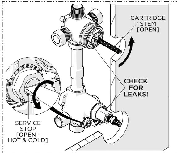
12. OPEN the SERVICE STOPS (hot & cold) and check for leaks. If no leaks are found, proceed and open the VOLUME CONTROL VALVE.
