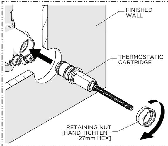
3. Insert the THERMOSTATIC CARTRIDGE into the VALVE BODY then thread and **hand-tighten** the RETAINING NUT into the VALVE BODY.
