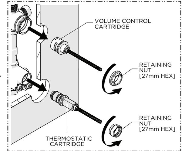
8. Unthread both RETAINING NUTS and remove both CARTRIDGES.
