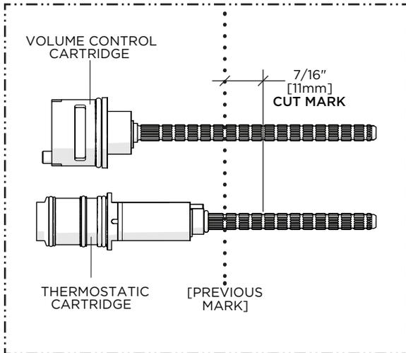
9. Carefully cut both CARTRIDGE STEMS 7/16" [11mm] in front of the previous mark so the STEMS will protrude 7/16" [11mm] from the finished wall surface.
