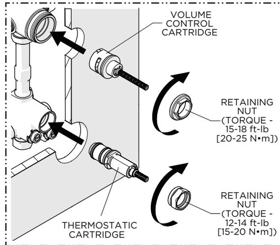
10. Insert both CARTRIDGES back into the VALVE BODY then thread and **securely** tighten the RETAINING NUTS to the specified torque settings shown.
