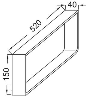
Product Specification: Towel rail bracket. EB507. Collection: PARALLEL. DIMENSIONS: 52 x 4 x 15 cm. WEIGHT: 1 kg. MATERIAL: Metal. INSTALLATION TYPE: Wall-hung. IMPORTANT: Towel rail bracket sold individually. Brushed metal.
