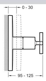
Product Specification: 3 + 3-way built-in diverter - Classic trim. E75415. Collection: MODULO. DIMENSIONS: 18 x 14 cm. WEIGHT: 2 kg. MATERIAL: Metal. INSTALLATION TYPE: Wall-mount.
