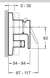
Product Specification: Two-way shower mixer, Strayt trim and lever. E98633. Collection: STRAYT. DIMENSIONS: 16.60 x 13.50 cm. WEIGHT: 2.8 kg. MATERIAL: Metal. INSTALLATION TYPE: Built-in. NORMS AND REGULATION: ACS (Certificate of Sanitary Compliance): 10 ACC LY 004. COMPONENTS: Build-in body, trim and handle. CONNECTIONS: Connect to two outlets (example: showerhead, handshower, bath spout).
