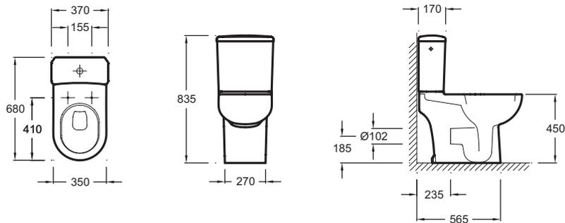
Product Specification: Raised WC pack PRM, vario outlet. E8353. Collection: ODÉON. DIMENSIONS: 68 x 35 cm. WEIGHT: 44.2 kg. MATERIAL: Ceramic. INSTALLATION TYPE: Floor-standing. NORMS AND REGULATION: NF. VOLUME OF WATER: Standard 3/6 L. HEIGHT: Surélevée/PMR. RIM TYPE: Open (traditional). SUPPLIED WITH: Thermoset seat, adjustable stainless steel hinges E4750 ; 2 floor fixings kits. Side inlet.
