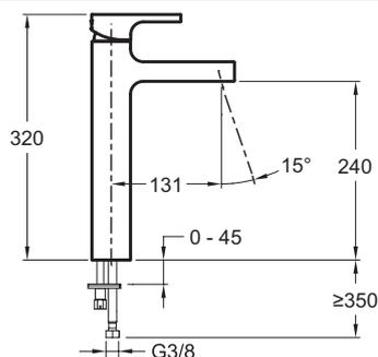
Product Specification: Tall single-lever washbasin mixer, smooth body. E98340. Collection: STRAYT. WEIGHT: 4.2 kg. MATERIAL: Metal. INSTALLATION TYPE: 1 hole. TYPE: Single-lever. FLOW RATE: 5 l/min. CONNECTION: With supply hoses. WASTE : Without waste. INSTALLATION TYPE: 1 hole. MECHANISM GUARANTEE: 5 years. No waste.
