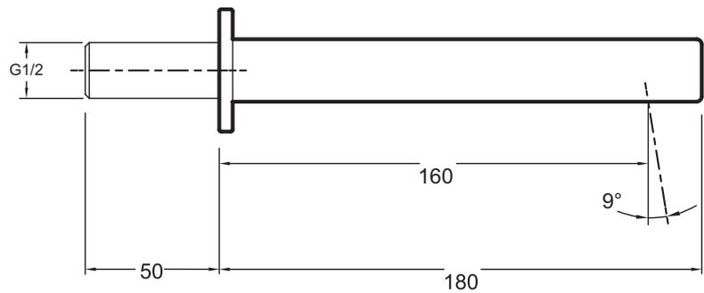
Product Specification: Wall-mount bath filler, E37344. Collection: STRAYT. WEIGHT: 1 kg. MATERIAL: Metal. INSTALLATION TYPE: Wall-mount. FLOW RATE: 30 l/min. SPOUT PROJECTION: 180.
