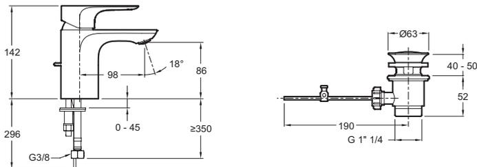
Product Specification: Single-lever washbasin mixer with 5/35" system. E72275-4. Collection: ALEO. WEIGHT: 1.4 kg. MATERIAL: Metal. INSTALLATION TYPE: 1 hole. NORMS AND REGULATION: NF : I - ECAU : E00 Ch2 A3 U3 (Ps3) - ACS : 10 ACCLY 113. TYPE: Single-lever. FLOW RATE: 5 l/mn. HEIGHT UNDER SPOUT: 142. SPOUT PROJECTION: 98. CONNECTION: With supply hoses. MECHANISM: Cartouche à disques céramique. WASTE : With waste. INSTALLATION TYPE: 1 hole. MECHANISM GUARANTEE: 5 years.
