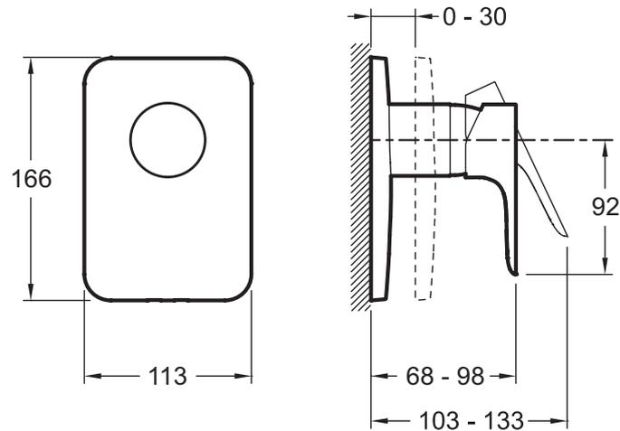
Product Specification: Built-in shower mixer, E98705. Collection: ALEO. DIMENSIONS: 24.50 x 16.50 x 11.50 cm. WEIGHT: 1.9 kg. MATERIAL: Metal. INSTALLATION TYPE: Built-in. NORMS AND REGULATION: Standards: ACS (Certificate of Sanitary Compliance):10 ACC LY 004. COMPONENTS: Build-in body, trim and handle. CONNECTION : Connect to an outlet (example: showerhead, handshower).
