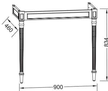
Product Specification: Washstand 90 cm. EB727. Collection: CLÉO 1889. DIMENSIONS: 90 x 46 x 83.40 cm. WEIGHT: 10 kg. MATERIAL: Lacquer. INSTALLATION TYPE: Floor-standing.
