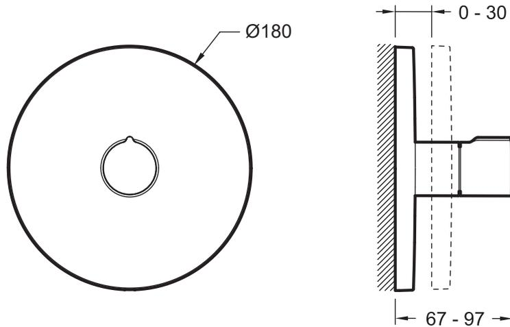
Product Specification: 3 + 3-way built-in diverter - Round trim. E19032. Collection: MODULO. WEIGHT: 2 kg. MATERIAL: Metal. INSTALLATION TYPE: Built-in. COMPONENTS: Build-in body, trim and Hybrid handle.
