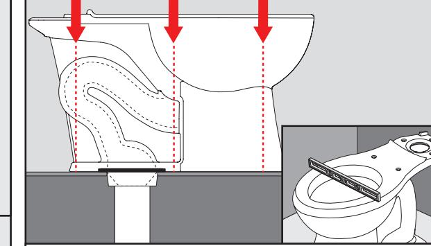
Carefully place toilet over the flange. Align horn and mounting holes on toilet with the wax ring and bolts on floor. Apply weight evenly until toilet is flush to the floor. **Do not move after placement or watertight seal may be broken.**
