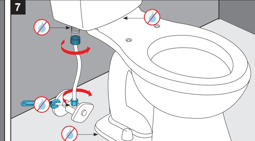
If optional fittings are included, remove or discard if not needed. **REMOVE AND DISCARD CARDBOARD INSIDE OF THE TANK.** Connect water supply line to the toilet and the water stop. Turn on water and flush the toilet several times. **Check for leaks.**
