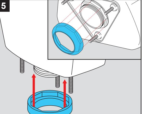
Place tank on the bowl and secure using the three washers and nuts.
