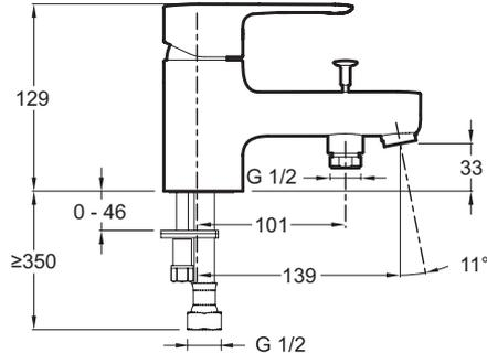
Product Specification: Single-lever bath/shower mixer. E16044-4. Collection: JULY. WEIGHT: 1.5 kg. MATERIAL: Metal. INSTALLATION TYPE: 1 hole. NORMS AND REGULATION: NF : IC/A - ECAU : E3/1 C2 A3 U3 - Ge3. TYPE: Single-lever. FLOW RATE: 21 l/min. CONNECTION: With pillar connectors. MECHANISM: Ceramic disc cartridge. WATER/ENERGY-SAVING: WATER-SAVING. WASTE : Without waste. DIVERTER: Automatic diverter with locking feature. MECHANISM GUARANTEE: 5 years. Anti-scale aerator.
