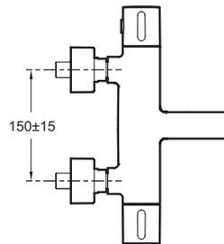
Product Specification: Single-lever thermostatic wall-mount bath/shower mixer. E78520. Collection: CUFF. MATERIAL: Metal. INSTALLATION TYPE: 2 holes. NORMS AND REGULATION: NF : II\*/A - ECAU : E3/1 C3 A1 U3 - ACS : 10 ACCLY 103. TYPE: Single-lever. FLOW RATE: 20 l/mn. CONNECTION: With connectors and wall escutcheons. WATER/ENERGY-SAVING: WATER-SAVING. SAFETY STOP: 38°C. DIVERTER: Automatic diverter built into flow handle. MECHANISM GUARANTEE: 5 years. Warm body: compartmentalized interior.
