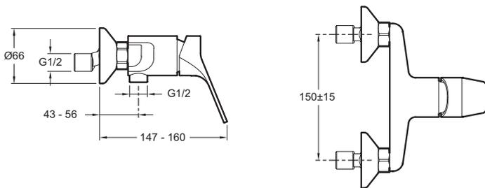
Product Specification: Single-lever wall shower mixer. E75765. Collection: BRIVE. WEIGHT: 1 kg. MATERIAL: Metal. INSTALLATION TYPE: 2 holes. NORMS AND REGULATION: NF : IA - ECAU : E1 C2 A2 U3 (Ge3) - ACS : 15 ACC LY 472. TYPE: Single-lever. FLOW RATE: 13 l/mn. CONNECTION: With connectors and wall escutcheons. MECHANISM: Ceramic disc cartridge. HOLE CONFIGURATION:  $150 \pm 15$ . MECHANISM GUARANTEE: 5 years. Non-return valve on shower outlet.
