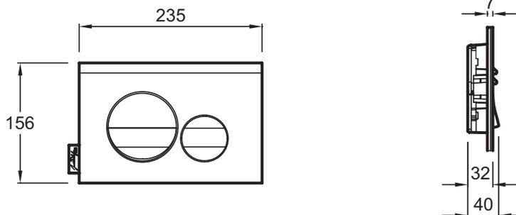
Product Specification: Flush plate, round pushbuttons. E20859. Collection: NO COLLECTION. DIMENSIONS: 23.50 x 15.60 cm. WEIGHT: 0.5 kg. MATERIAL: 54. INSTALLATION TYPE: Wall-mount. SINGLE/DUAL FLUSH: Dual flush. SEAT : Not included. Dual flush.
