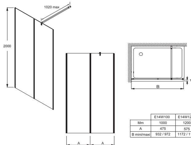
Product Specification: Fixed side panel 100 cm. E14W100. Collection: SERENITY. DIMENSIONS: 200 x 0.60 cm. WEIGHT: 32 kg. MATERIAL: Clear glass. INSTALLATION TYPE: Walk-in. NORMS AND REGULATION: EN 14428. REINFORCING BAR: horizontal, included with the fixed panel. GLASS THICKNESS IN MM: 6. PANEL HEIGHT IN CM: 200. ENCLOSURE TYPE: Walk-in. INSTALLATION: Open Space. ANTI-SCALE TREATMENT: Yes.
