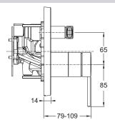
Product Specification: Built-in mechanical mixer. E78021-4A. Collection: MÉTRO. MATERIAL: Metal. INSTALLATION TYPE: Built-in.
