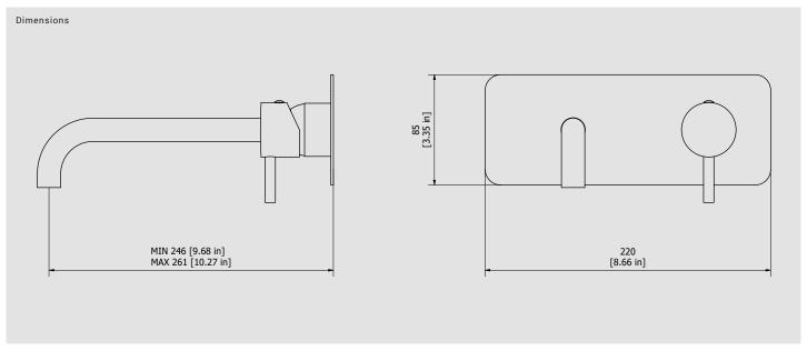
Cartridge Threaded fitting G1/2" female Ø35 ceramic cartridge Aerator Flow Rate (+/-10%) 1 BAR 2 BAR 3 BAR M16.5x1 3 I\m 3.8 l\m 3.8 I\m
