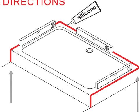
Ensure the shower tray is level in all directions and is properly sealed to the wall. The wall must be tiled down to the top edge of the tray. **Do not angle out bottom tile.**
