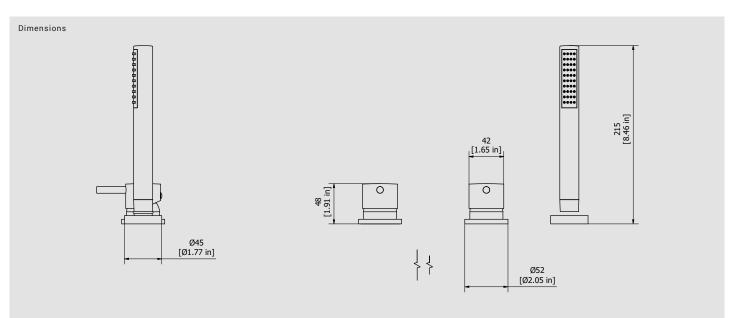
Cartridge Treaded fitting Inox hoses G1/2" F L300 Ø35 ceramic cartridge Aerator Flow Rate (+/-10%) 1 BAR 2 BAR 3 BAR M24x1 12 I\m 17 I\m 22 I\m
