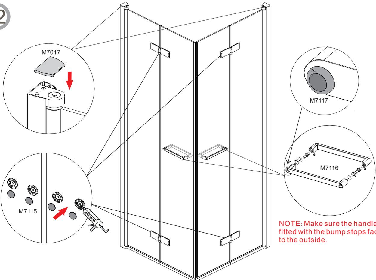
**NOTE:** Make sure the handle is fitted with the bump stops facing to the outside.
