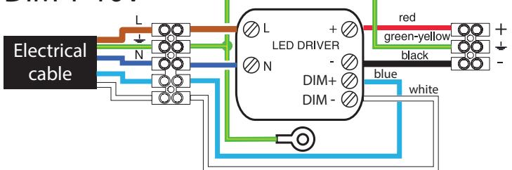
**EN** Connect the lamp to the mains according to the wiring diagram.
