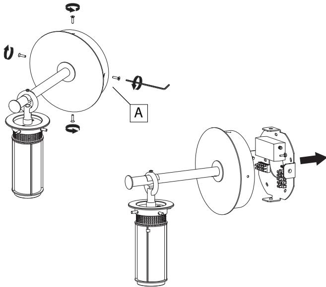
**EN** Unfasten the screws (A) that hold the rose to wall mounting bracket. Ensure the power is turned off at main circuit breaker and wall switch. Using the wall mounting bracket as a template, mark the positioning of the holes to be drilled in the wall for fixation of the lamp, and once satisfied with the positioning, proceed with drilling the holes. Install the screw anchors (B) supplied, and then fasten the bracket to the wall using screws (C).
