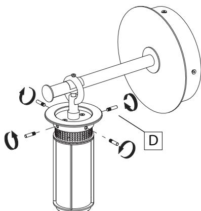
**EN** Unfasten the headless screws (D). From the main body. Install the diffuser and then re-fasten the screws (D) to secure it. Remove the locking screw and protecting piece (E).
