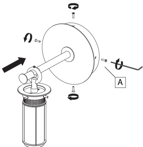
**EN** Fit the rose to wall mounting bracket and fasten the screws (A).
