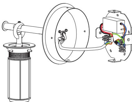
**EN** Make the electrical connections to the lamp as shown in the diagram.
