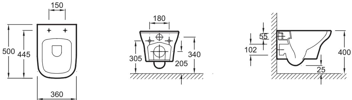
Product Specification: Rimless wall-hung WC pan. EDM102. Collection: VOX. DIMENSIONS: 50 x 36 cm. WEIGHT: 21.2 kg. MATERIAL: Ceramic. INSTALLATION TYPE: Wall-hung. VOLUME OF WATER: Standard 3/6 L. RIM TYPE: Rimless. RIM: Without rim. PRODUCT INCLUDED: (Seat not included). SEAT : Not included. TOILET BOWL FIXINGS: Invisible.
