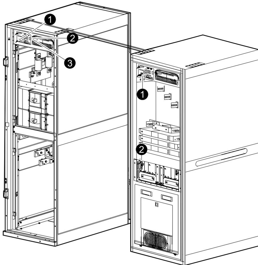
1. Connect the cable 0W3759 from connector J6500 on 0P4739 the I/O cabinet to connector J6500 on 0P4739 in the battery breaker cabinet. Attach the cable to the cable relief in the lower left corner.
