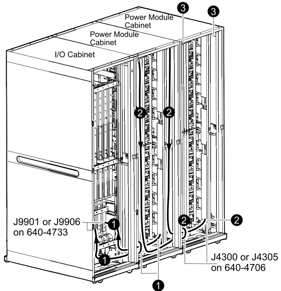
1. Locate the MIM/RIM cables that are placed in the bottom of the power module cabinet next to the I/O cabinet and connect them in the bottom of the I/O cabinet (left to left and right to right).
