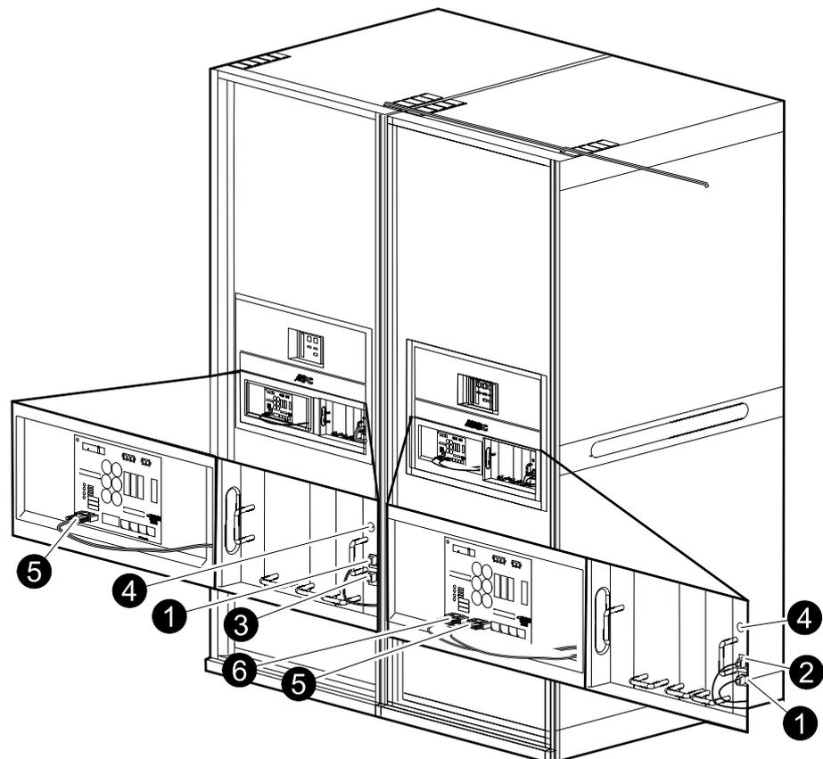
1. Remove the terminator from the bottom Abus terminal on the battery cabinet that is connected to the I/O cabinet. Connect the cable 0W4527 from the Abus terminal to the top Abus terminal in the next battery cabinet.
