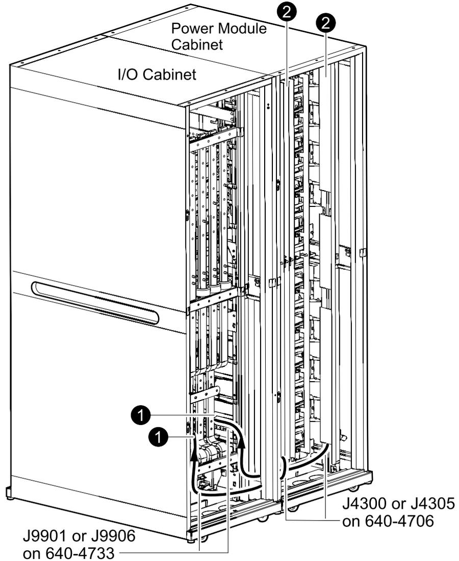
1. Locate the MIM/RIM cables that are placed in the bottom of the power module cabinet and connect them in the bottom of the I/O cabinet (left to left and right to right).
