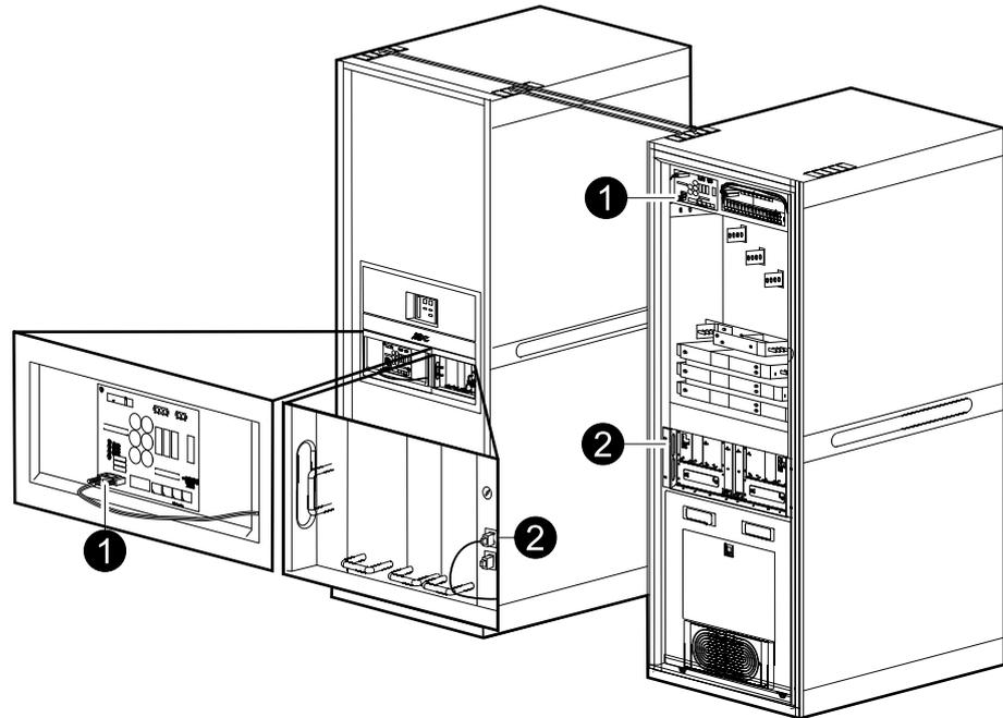
1. Connect the cable 0W4528 (0W3759 in installations with remote batteries) from connector J6500 on 0P4711 in the I/O cabinet to connector J6500 on 0P4711 in the battery cabinet.
