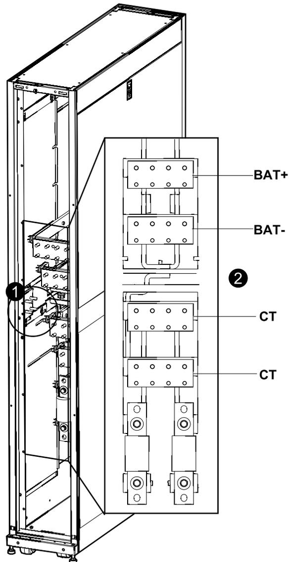
2. Connect one end of the battery cables to the BAT+, BAT-, and CT (Midpoint) cable landings in the battery side car.
