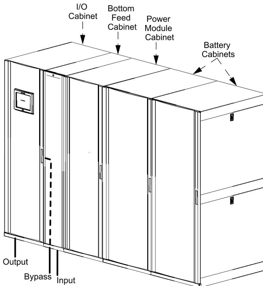
In systems with bottom cable entry, the input and bypass cables are routed through the bottom of the bottom feed cabinet. The output cables are routed through the bottom of the I/O cabinet.
