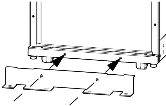
3. Push the cabinet backwards so the rear anchoring bracket on the cabinet slides under the floor anchoring bracket.
