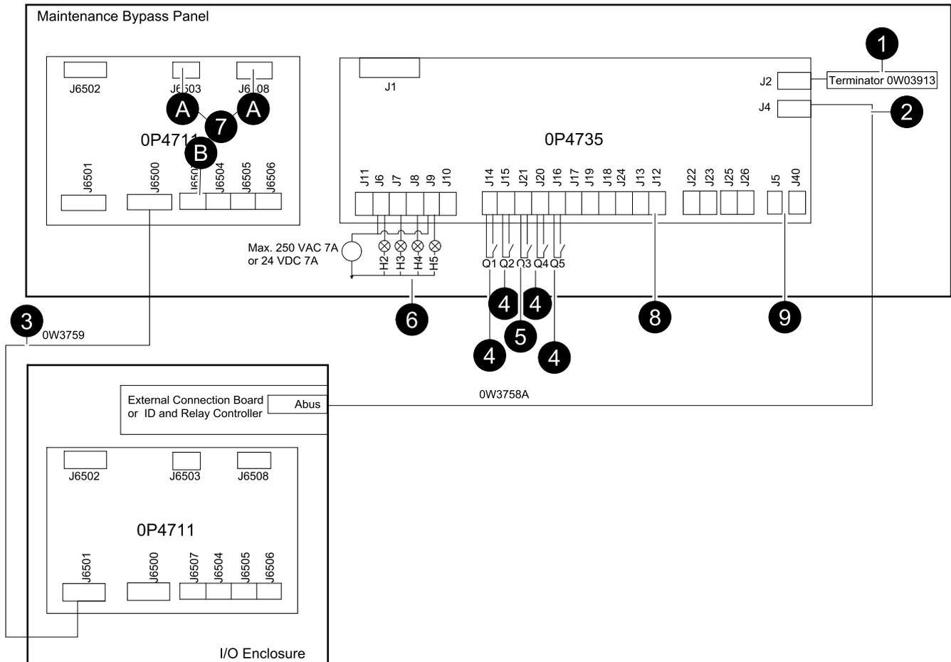
1. Install terminator 0W03913 in the J2 terminal on the OP4735.
