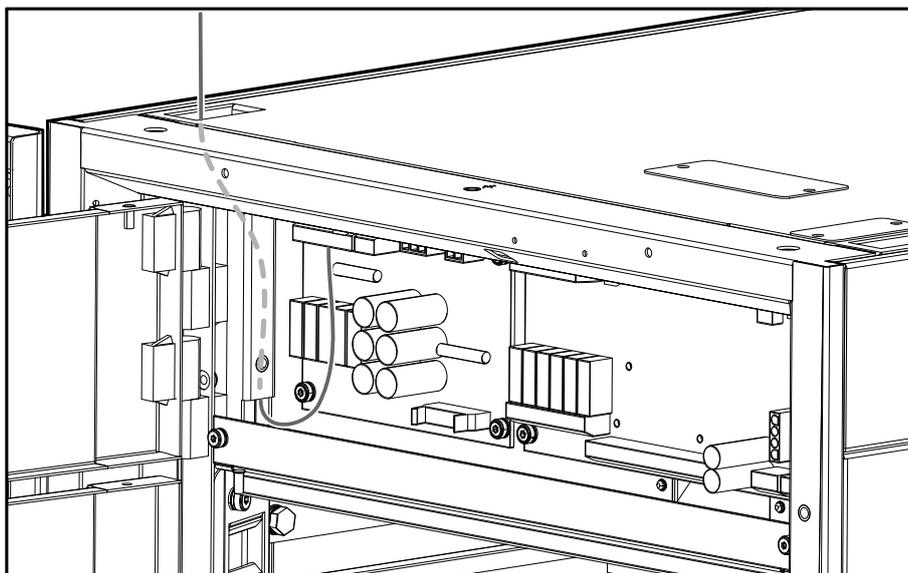
3. Connect the cable from the EPO to the EPO connection and trip board. A normally open installation is shown.
