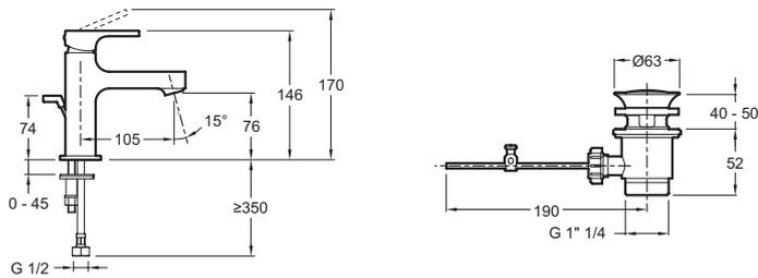
Product Specification: Standard single-lever washbasin mixer with supply hoses. E8776. Collection: STRAYT. WEIGHT: 1.6 kg. MATERIAL: Metal. INSTALLATION TYPE: 1 hole. NORMS AND REGULATION: ACS : 14 ACC LY 511. TYPE: Single-lever. FLOW RATE: 5 l/mn. HEIGHT UNDER SPOUT: 146. SPOUT PROJECTION: 105. CONNECTION: With supply hoses. MECHANISM: Cartouche à disques céramique. INSTALLATION TYPE: 1 hole. MECHANISM GUARANTEE: 5 years. Metal waste. Anti-scale aerator.
