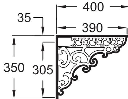
Product Specification: Pair of fixing brackets. E26370. Collection: CLÉO 1889. WEIGHT: 1.1 kg. MATERIAL: Cast iron.
