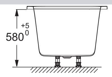
Product Specification: Front and end panel. E6D133. Collection: PANOLUX. DIMENSIONS: 140 x 90 x 58 cm. WEIGHT: 11 kg. MATERIAL: Panolux. INSTALLATION TYPE: Corner. INSTALLATION: Aprons for alcove or corner installation. Cut to size for Capsule 120 x 80 cm..
