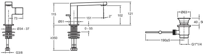
Product Specification: Single-lever washbasin mixer - "Pure" lever. E73050. Collection: COMPOSED. WEIGHT: 2.5 kg. MATERIAL: Metal. INSTALLATION TYPE: 1 hole. NORMS AND REGULATION: ACS : 14CCLY511. TYPE: Single-lever. FLOW RATE: Maximum flow 5 l/min. HEIGHT UNDER SPOUT: 121. SPOUT PROJECTION: 151. CONNECTION: With supply hoses. MECHANISM: Ceramic disc cartridge. WATER/ENERGY-SAVING: WATER-SAVING. WASTE : With waste. INSTALLATION TYPE: 1 hole. MECHANISM GUARANTEE: 5 years. Anti-scale aerator.
