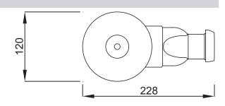
Product Specification: Extra-slim waste. E78168. Collection: NO COLLECTION. WEIGHT: 0.3 kg. MATERIAL: 54. INSTALLATION TYPE: 38. WASTE DIAMETER: 9 cm. Flow rate: 36 L/ min.
