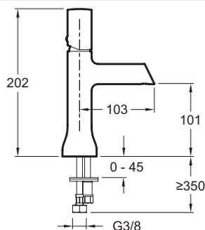
Product Specification: Single-lever washbasin mixer, smooth body. E7329. Collection: TOOBI. WEIGHT: 1.3 kg. MATERIAL: Metal. INSTALLATION TYPE: 1 hole. TYPE: Single-lever. FLOW RATE: 5 l/min. CONNECTION: With supply hoses. MECHANISM: Ceramic disc cartridge. WASTE : Without waste. INSTALLATION TYPE: 1 hole. MECHANISM GUARANTEE: 5 years. Flow up to 8 l/mn. No waste.
