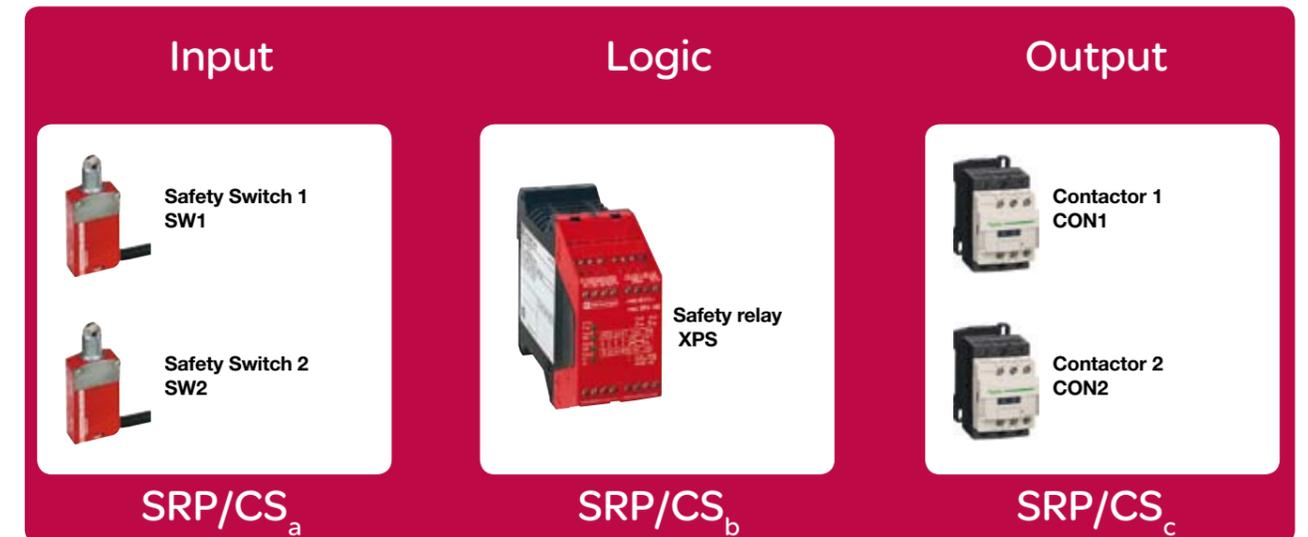
> STEP 4: The PL of the SRP/CS is determined by estimation of the following parameters: (see Annex 2):
