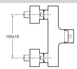
Product Specification: Single-lever wall shower mixer. E45371. Collection: STRAYT. WEIGHT: 3.7 kg. MATERIAL: Metal. INSTALLATION TYPE: 2 holes. TYPE: Single-lever. CONNECTION: With connectors and wall escutcheons. MECHANISM: Ceramix disc cartridge. MECHANISM GUARANTEE: 5 years. Water saving feature. Connectors with wall escutcheons. Non-return valve on shower outlet.
