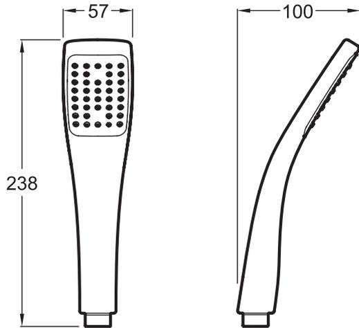
Product Specification: Handshower - Small. E3876. Collection: EO. DIMENSIONS: 6 x 10 x 24 cm. MATERIAL: Metal. INSTALLATION TYPE: Wall-mount. 38 nozzles.
