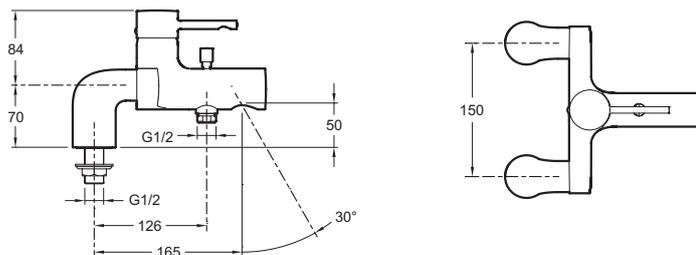
Product Specification: Single-lever deck-mount bath/shower mixer. E37043. Collection: CUFF. WEIGHT: 3 kg. MATERIAL: 54. INSTALLATION TYPE: 2 holes. NORMS AND REGULATION: NF : IC/A - ECAU : E3/1 C2 A2 U3 - ACS : 10 ACC LY 004. TYPE: Single-lever. FLOW RATE: 20 l/min. CONNECTION: With pillar connectors. MECHANISM: Ceramic disc cartridge. HOLE CONFIGURATION: 150. DIVERTER: Automatic diverter with locking feature. MECHANISM GUARANTEE: 5 years.
