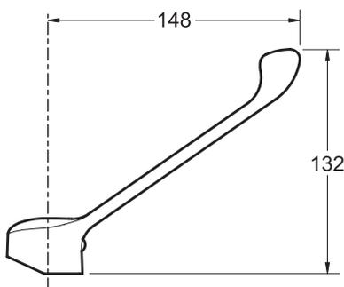
Product Specification: Elbow-control lever. E18164. Collection: EASY. MATERIAL: Metal. Long elbow-operated lever.
