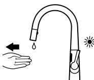
When the red LED of sensor starts to blink, remove hand. The water flow will stop, if it was open.
