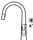
The LED blinks one time. Wait 5 sec. to start the adjustment process.
