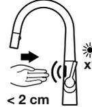
After 3 sec. the faucet starts water flow and the red LED blinks 1 time per sec. during 5 sec. Within those 5 sec. place hand in front of sensor closer than 2cm. The red LED remains lit and the water flow stops.
