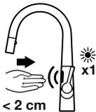
After 5 sec. the red LED turns off and the detection distance is set to the new value (2-10cm). If the hand is not placed or if it was removed from the sensor before 5 seconds, the faucet will be set to the longest detection distance (10cm).
