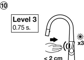
The LED blinks 3 times per sec. for 5 sec. To set Level 3 (0.75 sec.), place hand closer to 2 cm. from sensor. If this is not the desired adjustment, do not place hand.
