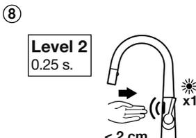
The LED blinks 1 time per sec. for 5 sec. To set Level 1 (0.25 sec.), place hand closer to 2 cm. from sensor. If this is not the desired adjustment, do not place hand.
