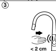
Place hand in front of the sensor closer than 2cm. for 5 sec. regardless of water flow .
