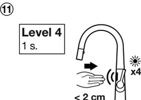
The LED blinks 4 times per sec. for 5 sec. To set Level 4 (1 sec.), place hand closer to 2 cm. from sensor. If this is not the desired adjustment, do not place hand.
