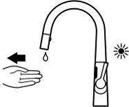
When the red LED of sensor starts to blink, remove hand. The water flow will stop, if it was open.
