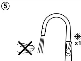
After 3 sec. the faucet starts water flow and the LED blinks 1 time per sec. during 5 sec. Do not place hand in front of sensor.
