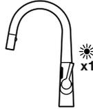
The LED blinks one time. Wait 5 sec. to start the adjustment process.
