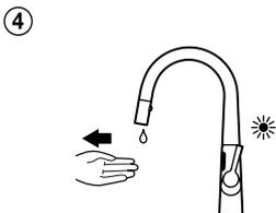
When the red LED of sensor starts to blink, remove hand. The water flow will stop, if it was open.
