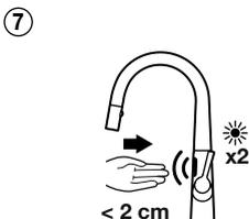
The faucet starts water flow and the LED blinks 2 times per sec. for 5 sec. within those 5 sec. place hand closer than 2 cm. The LED stops blinking and water flow stops. Remove hand before 3 sec.
