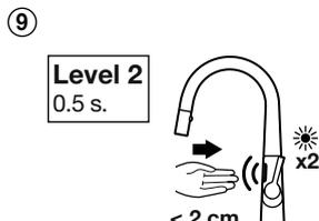
The LED blinks 2 times per sec. for 5 sec. To set Level 2 (0.5 sec.), place hand closer to 2 cm. from sensor. If this is not the desired adjustment, do not place hand.
