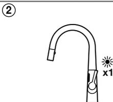
The LED blinks one time. Wait 5 sec. to start the adjustment process.
