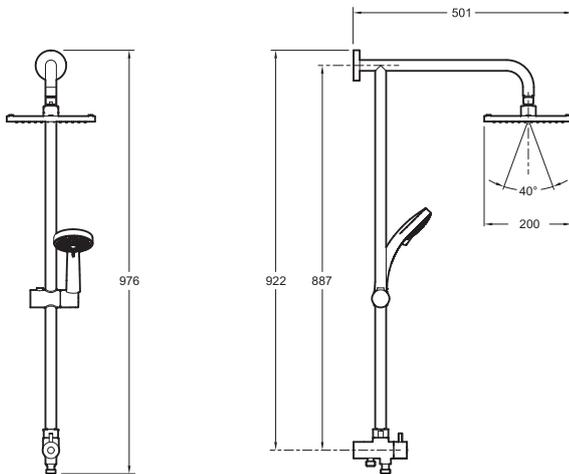
Product Specification: Shower column. E45893. Collection: EO. WEIGHT: 3 kg. MATERIAL: Metal. INSTALLATION TYPE: Wall-mount. WITH OR WITHOUT BRASSWARE: WITHOUT TAPS AND FITTINGS. SINGLE-LEVER TAPS: THERMOSTATIC.
