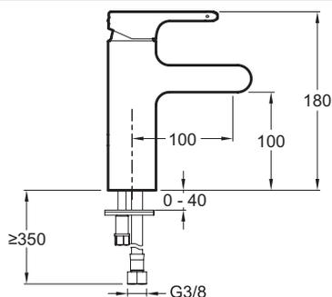
Product Specification: Single-lever basin mixer. E10496. Collection: SINGULIER. WEIGHT: 2.5 kg. MATERIAL: Metal. INSTALLATION TYPE: 1 hole. NORMS AND REGULATION: NF : I - ECAU : E1 C2 A2 U3. TYPE: Single-lever. FLOW RATE: 12 l/min. CONNECTION: With supply hoses. MECHANISM: Ceramic disc cartridge. HOLE CONFIGURATION: 180. WASTE : Without waste. MECHANISM GUARANTEE: 5 years.
