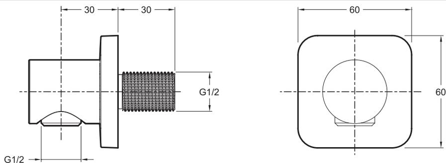
Product Specification: Wall elbow - Hybrid plate. E8463. Collection: MODULO. DIMENSIONS: 13.50 x 9 x 6.50 cm. WEIGHT: 0.5 kg. MATERIAL: Metal. INSTALLATION TYPE: Wall-mount. With non-return valve.
