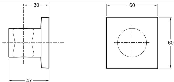
Product Specification: Wall handshower bracket - Square plate. 8468D. Collection: MODULO. DIMENSIONS: 13.50 x 9 x 6.50 cm. WEIGHT: 0.4 kg. MATERIAL: Metal. INSTALLATION TYPE: Wall-mount. Chromed brass.
